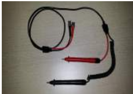
[Pin type battery test lead for impedance, voltage, temperature measurement]
